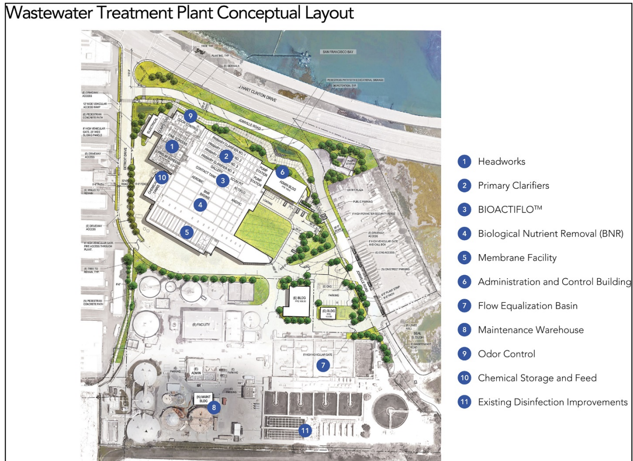
Figure 1 WWTP Conceptual Layout Displaying the Upgrade and Expansion of the WWTP in the Northern Half of the Site and the Existing WWTP Facilities in the Southern Half of the Site
